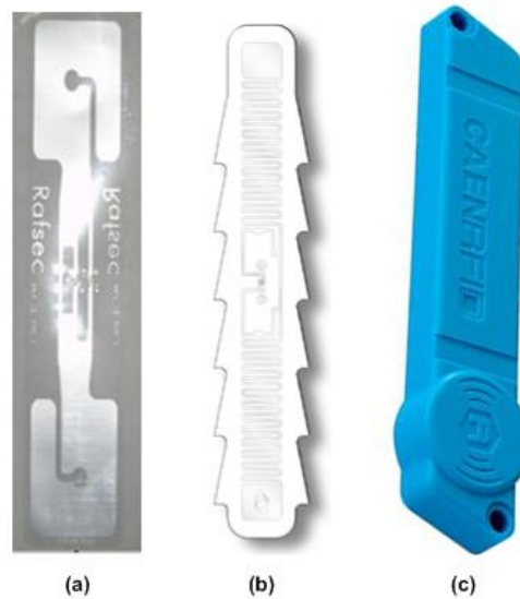
Figure 1. UHF RFID Tag Passive, special purpose and battery assisted.
